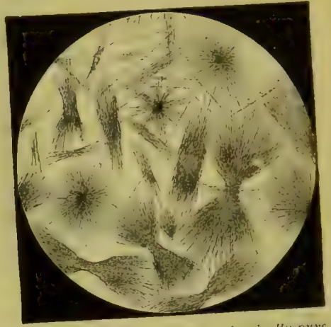
FIG. 121.—Lactate of lime, from chemically pure lactic acid and carbonate of lime, crystallized from a hot, watery solution. (Funke.)
